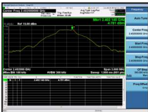
GFSK LOW CHANNEL, CARRIER LEVEL
