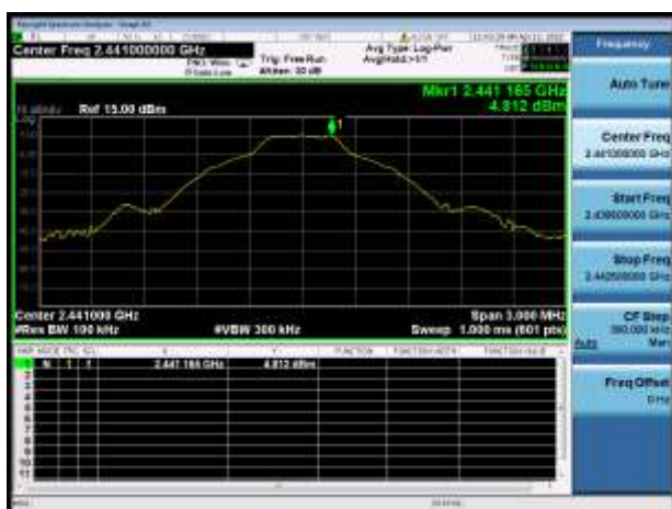
GFSK MIDDLE CHANNEL, CARRIER LEVEL
