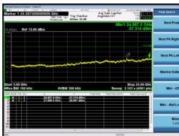
GFSK LOW CHANNEL, SPURIOUS 3 GHz ~ 25 GHz
