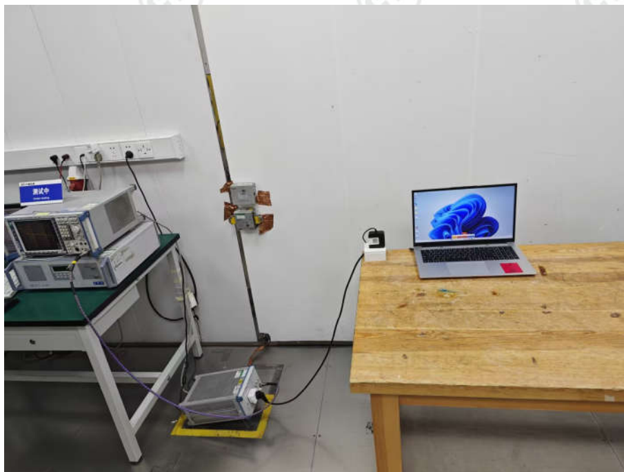
Conducted Emissions Test Setup
