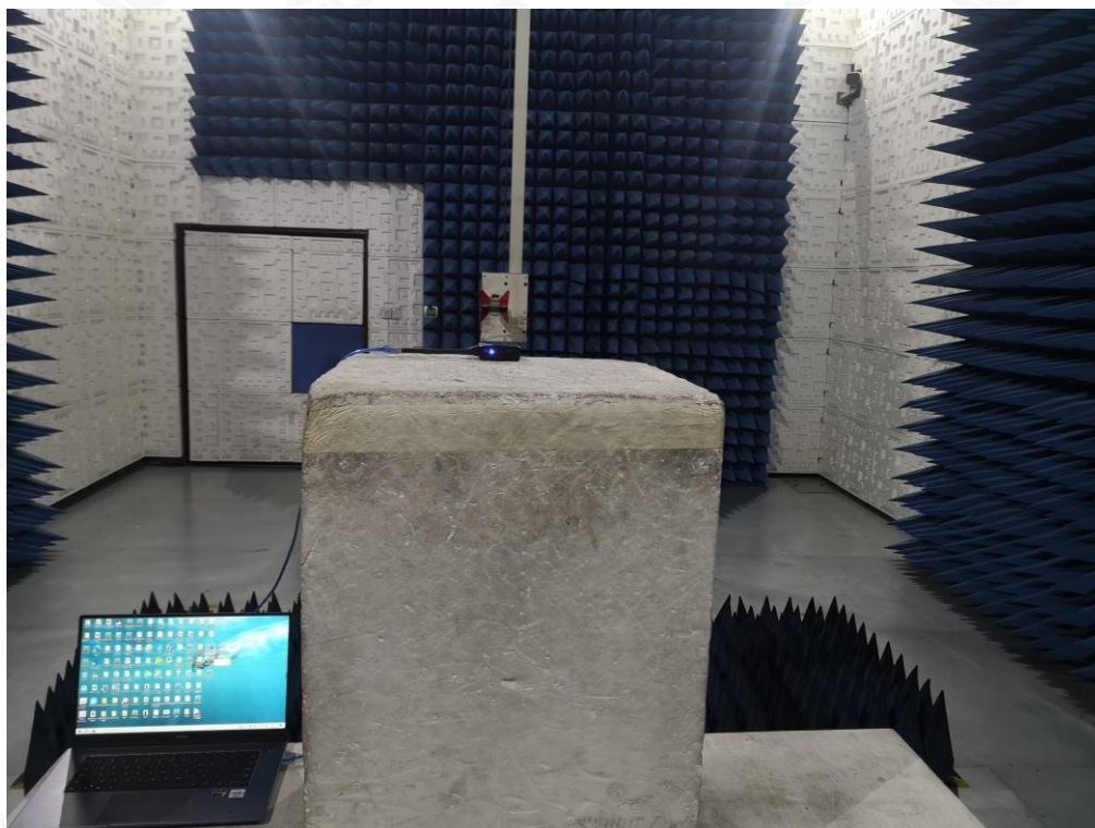
FCC RADIATED EMISSION TEST SETUP ABOVE 1GHZ
