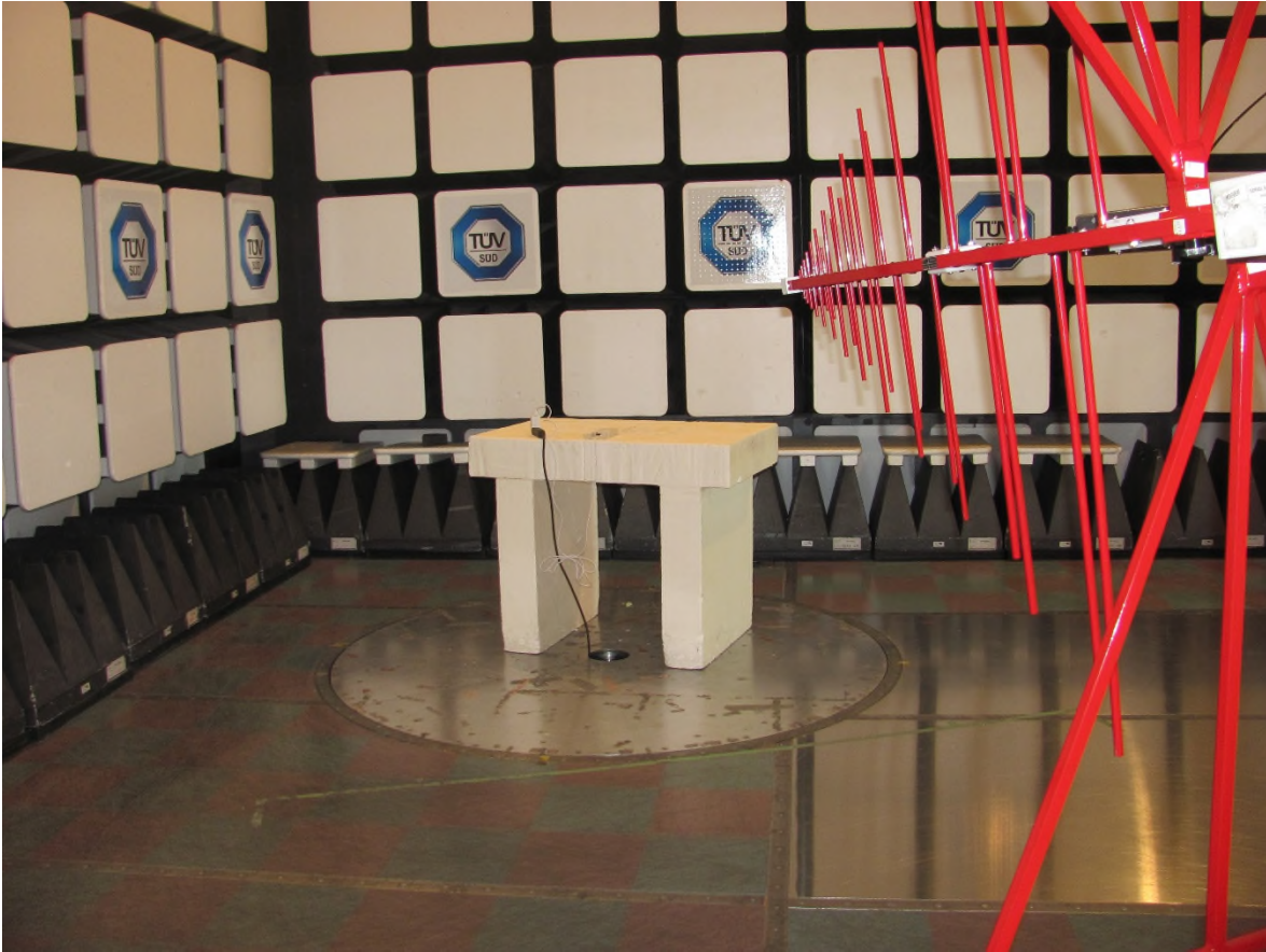
Figure 3 – Radiated Emissions Setup – Photo 3
