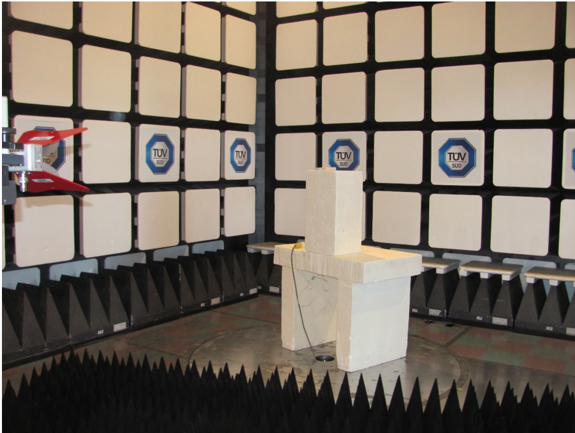
Figure 4 – Radiated Emissions Setup– Photo 4
