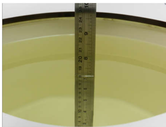
Fig 10.2 Photo of Liquid Height for Body SAR
