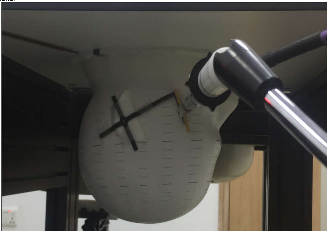
2.4GHz Dipole Placed at Location C in 90° Orientation (10mm Spacer)
