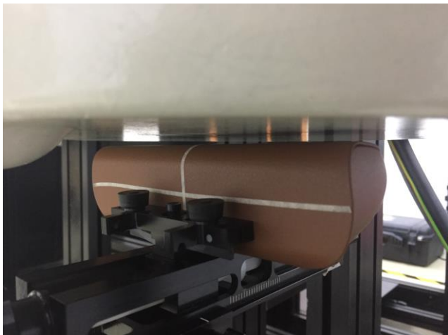
Bottom Edge Kept 5mm Distance from Phantom, Test Separation 5 mm
