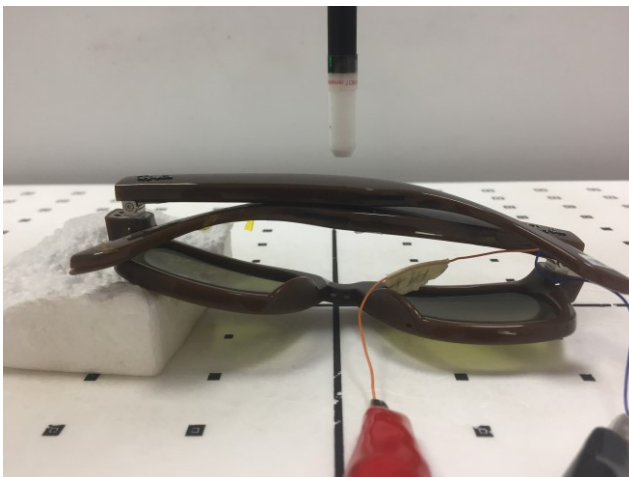
Left Temple Arm Outer Edge Touching Phantom, Test Separation 10 mm
