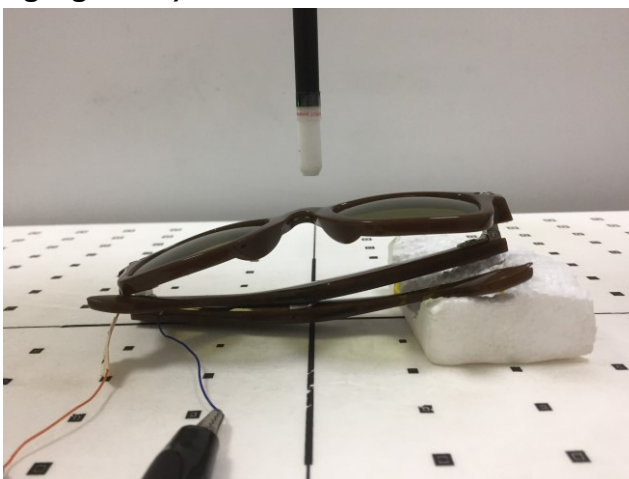
Left Lens Kept 5mm Distance from Phantom, Test Separation 10 mm
