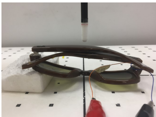
Left Temple Arm Outer Edge Touching Phantom, Test Separation 8.59 mm
