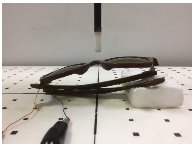
Left Lens Kept 5mm Distance from Phantom, Test Separation 8.59 mm
