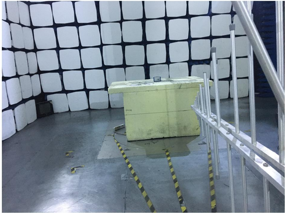
Radiation Emission Test Setup (30MHz to 1GHz)
