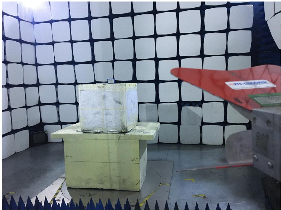
Radiation Emission Test Setup (1GHz to 18GHz)
