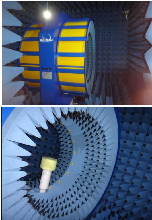
Imported from France's SATIMO StarLab 3D laboratory, it can accurately and quickly test the TRP, TIS, efficiency, gain, apple chart, directional chart and other parameter data of communication terminal products such as mobile phones, tablets and laptops.
