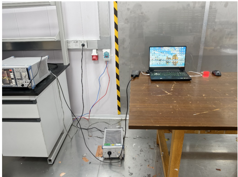
Conducted Emission Test Setup
