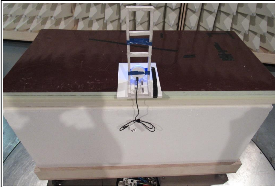
Test setup radiated emission EUT view 0.8m
