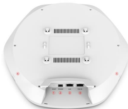
Figure 1-3 Physical interfaces of HS_C09961
