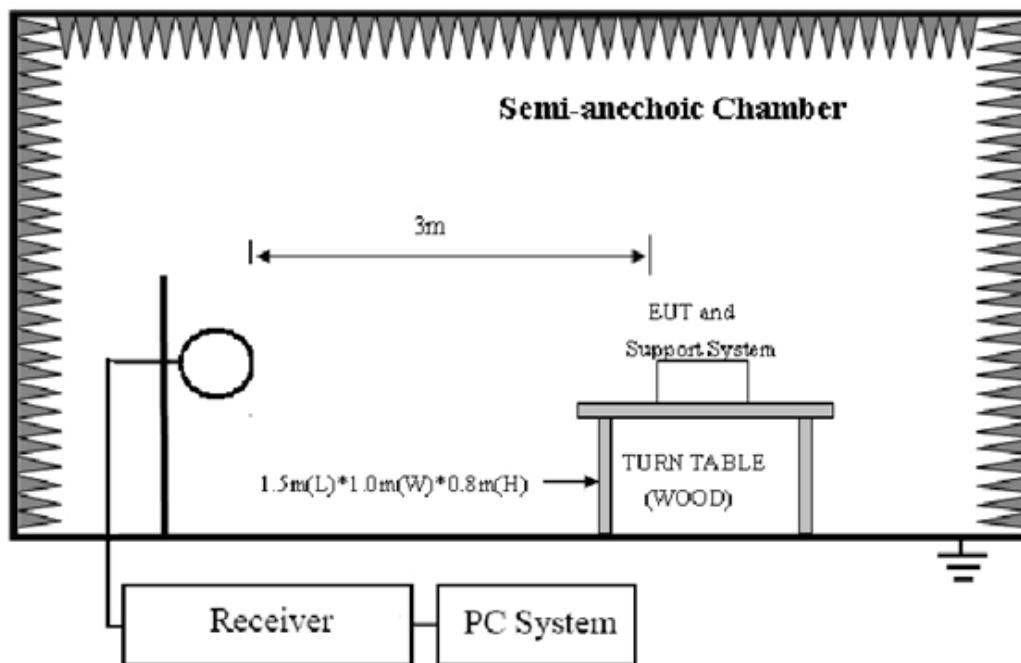
In 3m Anechoic Chamber Test Setup Diagram for 30MHz to 1GHz:
