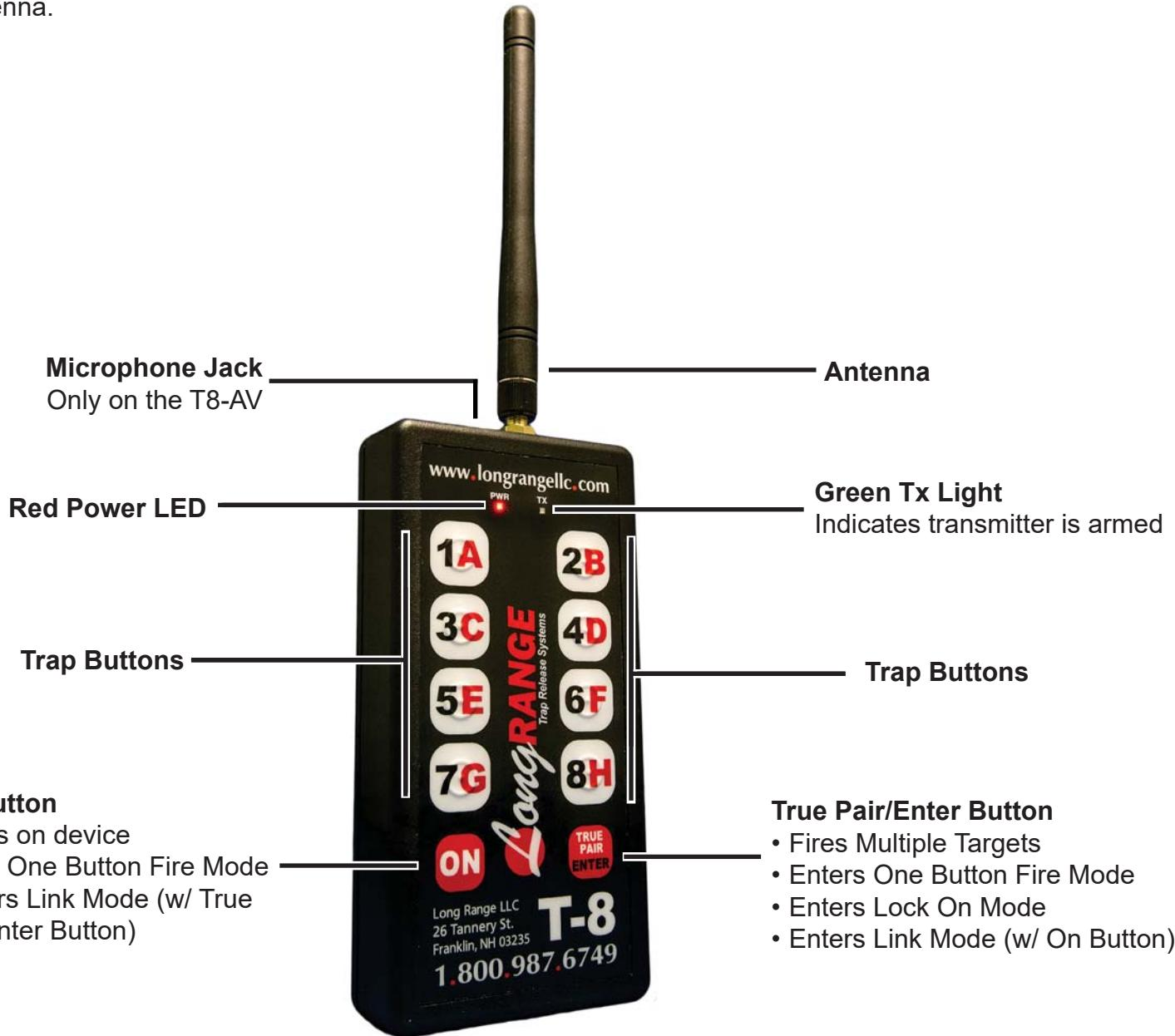
To turn on the transmitter, press the **On** button. The **Red Power LED** will illuminate to let you know that the device is on and ready to launch targets.
