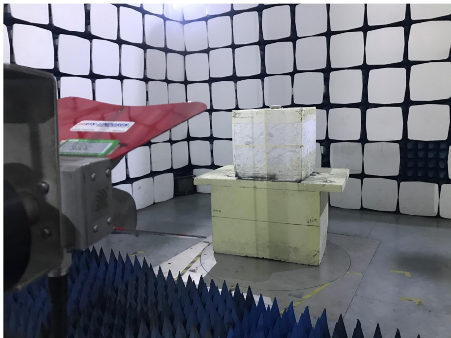
Radiation Emission Test Setup (1GHz to 18GHz)
