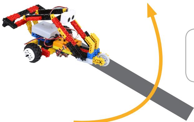
1. If the left infrared sensor is on the black line and the right infrared sensor is not on the black line, we will activate the right motor and turn it to the left.
