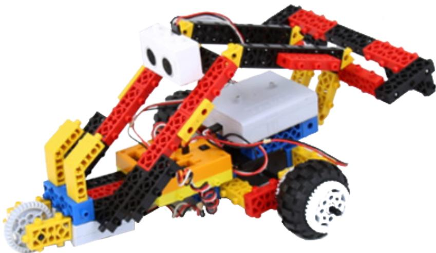
We will try to express motion by combining two infrared sensors, an input sensor, and an ultrasonic sensor and two DC motors. The two infrared sensors will continue to search for the black line. One of the remaining ultrasonic sensors stops working every time there are obstacle blocks. And if you get completely out of the black line, it will stop all operation.
