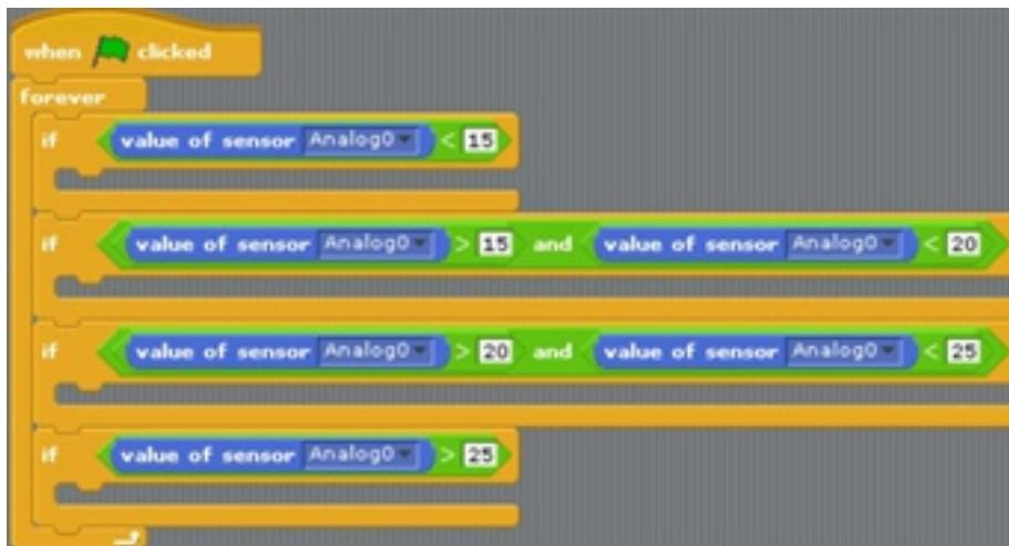
Did you make a script above? We split up the section using 'and' operator. Now let's put a coding block on how each LED sensor works in each section.
