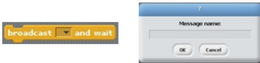
Click on the black arrow in the 'Broadcast and Wait' block to bring up the window shown above. In the 'Name of message' box, type the name of the script that will receive the signal. Make 'LED\_Shift' that will handle the operation of the LED sensor and 'Motor\_Move', which will be responsible for the operation of the motor.
