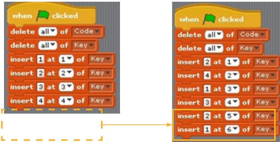
We can add two more blocks of 'input ~ to ~position of Key' to make my password six digits. You can pick 2 of the numbers from 1 to 4 and add them to positions 5,6 in the 'Key' list. Make your password six digits and see if the door of the safe works!
