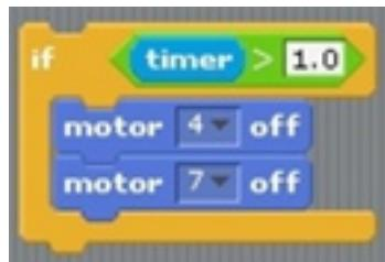
If the timer is greater than one second, I will stop the motor 4 and the motor 7. That is, if the input values of two infrared sensors do not come in conditionally, the time of the timer will continue to flow, and if the time exceeds 1 second (if the input value of the infrared sensor that does not meet the condition is kept over 1 second) It is.
