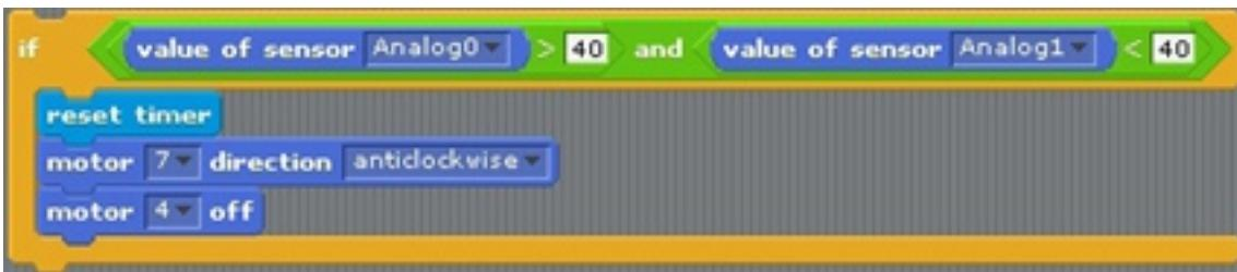
When you create the above script, the infrared sensor on the left is on the black line. When the infrared sensor on the right is not on the black line, the motor stops at 4, the 7 motor goes forward and the line tracer goes to the left. Now let's see how the left infrared sensor is not above the black line and the right infrared sensor is on the black line. Please create the script below.
