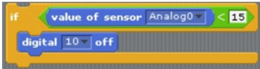
The above script will turn off the LED sensor connected to the digital 10 port when the ultrasonic sensor value is less than '15'. Now, when the ultrasonic sensor value is greater than '15', you have to turn on the LED sensor of digital 10 port. Please create the script below.
