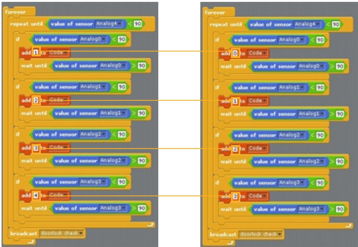
If you change only the numbers so that the input number is 0 ~ 3 instead of 1 ~ 4, the number of the button sensor changes from 0 ~ 3, so you can press '1003' to operate the door.
