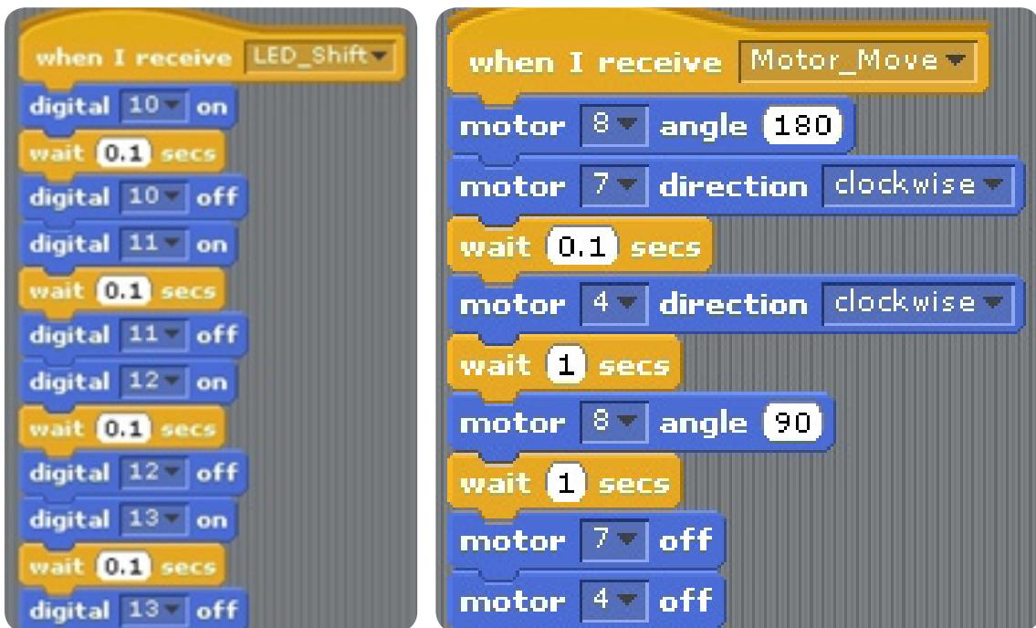
Does this script make sense? In the previous scripting with a single script, the length of the script was long and the distinction between each action was not clear. However, using the 'Broadcast' function makes it easier to create a script, and it makes good sense of the role of each script.
