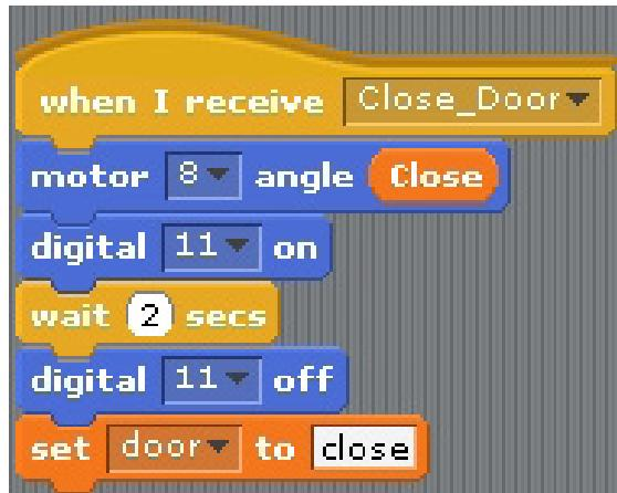
reate a script like the one above. First, close the door by activating the angle of motor No. 8 (servo motor) by the value stored in the 'Close' variable. After that, turn on Digital 11. (Turn on the sound sensor). After playing it for 2 seconds, turn off digital output 11 (turn off the sound sensor) and then store 'close' in the 'door' variable. The 'door' variable is a variable that indicates the current state of the statement.
