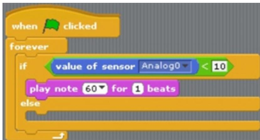
The above script is a script that will play a scale of 60 beats per minute if the distance between the ultrasonic sensor and the wall is less than '10'. The reason for using the 'if & else' syntax is that you have to play a different note if you are farther away from the analog value of the turtle '10'.
