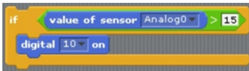
We created a script when the analog reference value is '15' above. When the remaining baseline values are '20' and '25', you can make the scripts the same. If analog reference value is '20', digital output 11 should be turned off and on. If analog reference value is '25', digital output 12 should be turned off and on. Once you've created each script, you can create a loop that will continue to check the condition with an 'infinite loop' block
