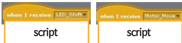
When 'LED\_Shift' or 'Motor\_Move' is broadcast, you have to receive the broadcast. The above picture is called 'When receiving LED\_Shift' and 'When receiving Motor\_Move'. And below that is the script that will be run after that. In other words, depending on which broadcast you have received, subsequent scripts will be executed. So we can create multiple scripts.
