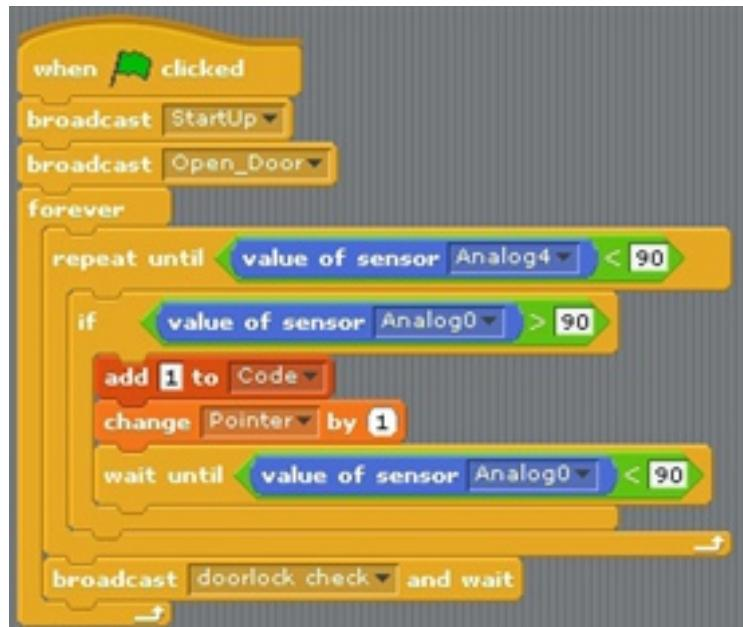
When you start the program, broadcast 'StartUp' and 'Open\_Door'. And there is one thing that changed: when you entered the number with the button sensor, and every time you enter the number, it accumulates the 'Pointer' variable. The reason to increase the 'Pointer' variable every time you press the sensor is to store the 'Pointer' value in the number of digits.
