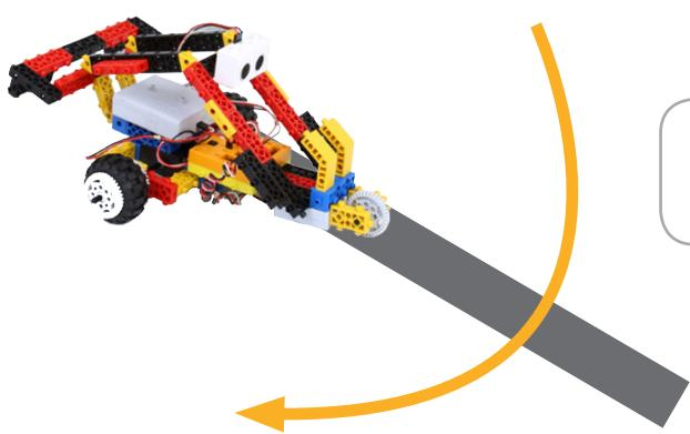
2. If the left infrared sensor is not on the black line and the right infrared sensor is on the black line, it will turn the left motor to the right.
