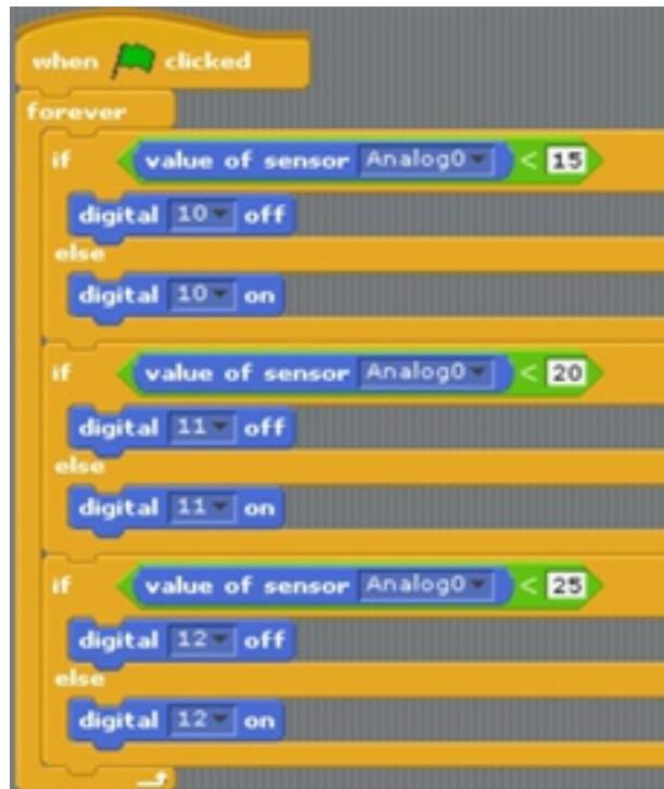
The script shown above now turns on the LED sensors one at a time as the distance from the wall increases. If the distance value is less than 15, all three LED sensors are turned off. If the distance value is greater than 15 and less than 20, one LED sensor is turned on (digital output 10 turns on) 'And less than' 25 ', two LED sensors are turned on, and if greater than' 25 ', three LED sensors are turned on.
