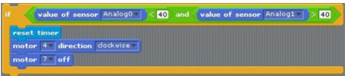
When you create the above script, the infrared sensor on the left is not on the black line. When the infrared sensor on the right is on the black line, motor 4 moves forward, stop motor 7, and let the line tracer go to the right. Now, let's create a script for an ultrasonic sensor. If the line tracer follows the black line and meets an obstacle, you must stop using the ultrasonic sensor.
