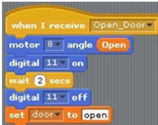
Create a script like the one above. First, open the door by activating the angle of motor 8 (servomotor) by the value stored in 'Open' variable. After that, turn on Digital 11. (Turn on the sound sensor.) Turn off Digital 11 output after playing for 2 seconds. (Turn off the sound sensor). And we store 'open' in the 'door' variable. The 'door' variable is a variable that tells you the current state of the statement.
