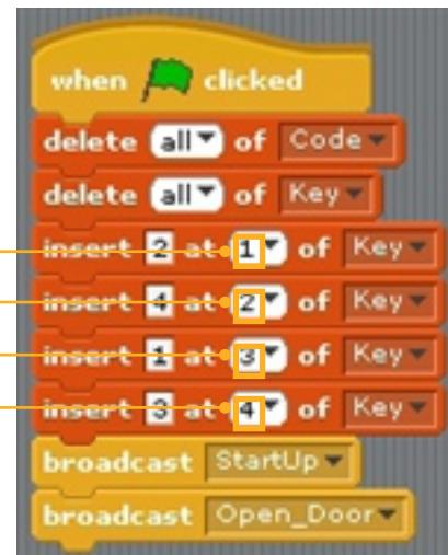
The above script puts '2', '4', '1', '3' in positions 1,2,3,4 of 'Key' list. If the existing items in the list are '1', '2', '3', or '4', just change the items in the list! Test that it works with the changed password!
