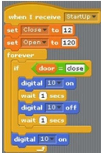
Create a script like the one above. 'Close' is the angle of the servo motor when the door is closed, and 'Open' is the angle of the servo motor when the door is opened. After setting the initial values of these two variables, try coding the operation of the LED sensor. The LED sensor will flash every 1 second if the door is closed and stay on if the door is open. The coding of the operation of the LED sensor will be discussed in detail on the next page.
