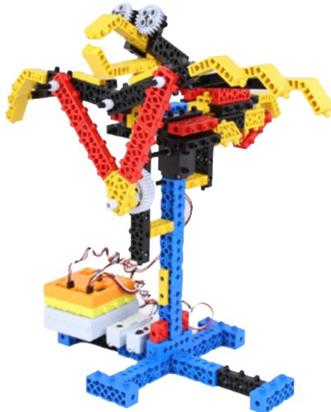
We are going to make it move by combining a input sensor-button sensor, a output sensor-sound sensor, and a DC motor. Let's make the wings flap and play music from the sound sensor whenever the button sensor is pressed.
