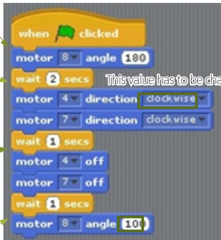
Type in an angle at which the tongs are closed.
