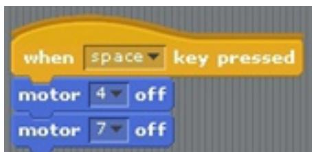
Tip: It will be easier to make the robot move if you make a code that stops Motor4 and Motor7 when the spacebar is pressed.
