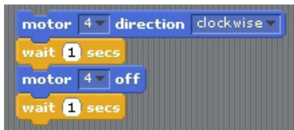
If you activate this, the left wheel of the lizard robot will turn on for 1 second and turn off.
