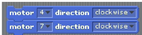
If you code following the picture above, the computer will activate Motor4 and Motor7 at the same time and move the robot forward.
