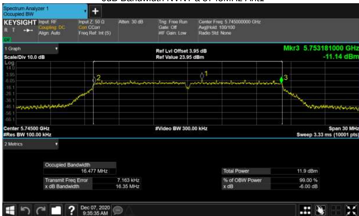
-6dB Bandwidth NVNT a 5745MHz Ant1
