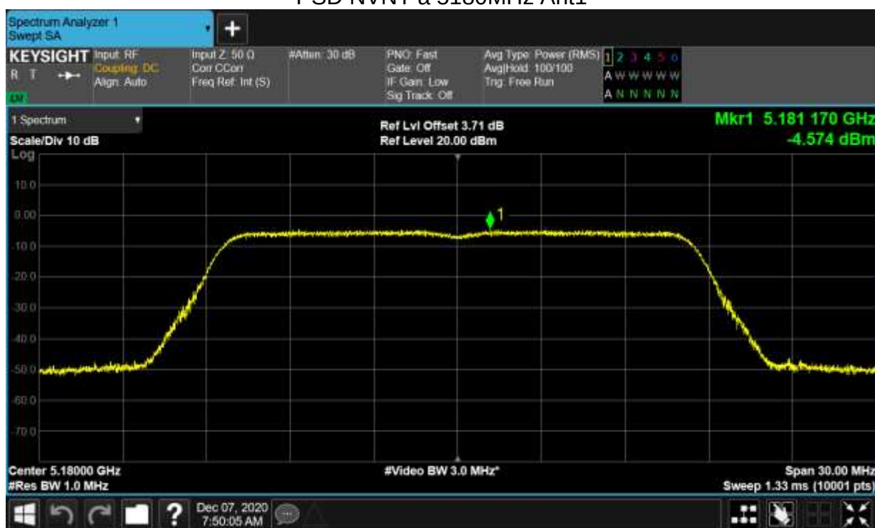
PSD NVNT a 5180MHz Ant1
