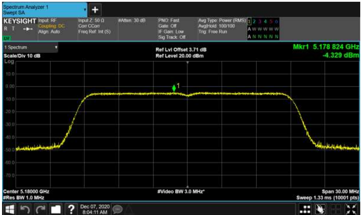
PSD NVNT n20 5180MHz Ant1
