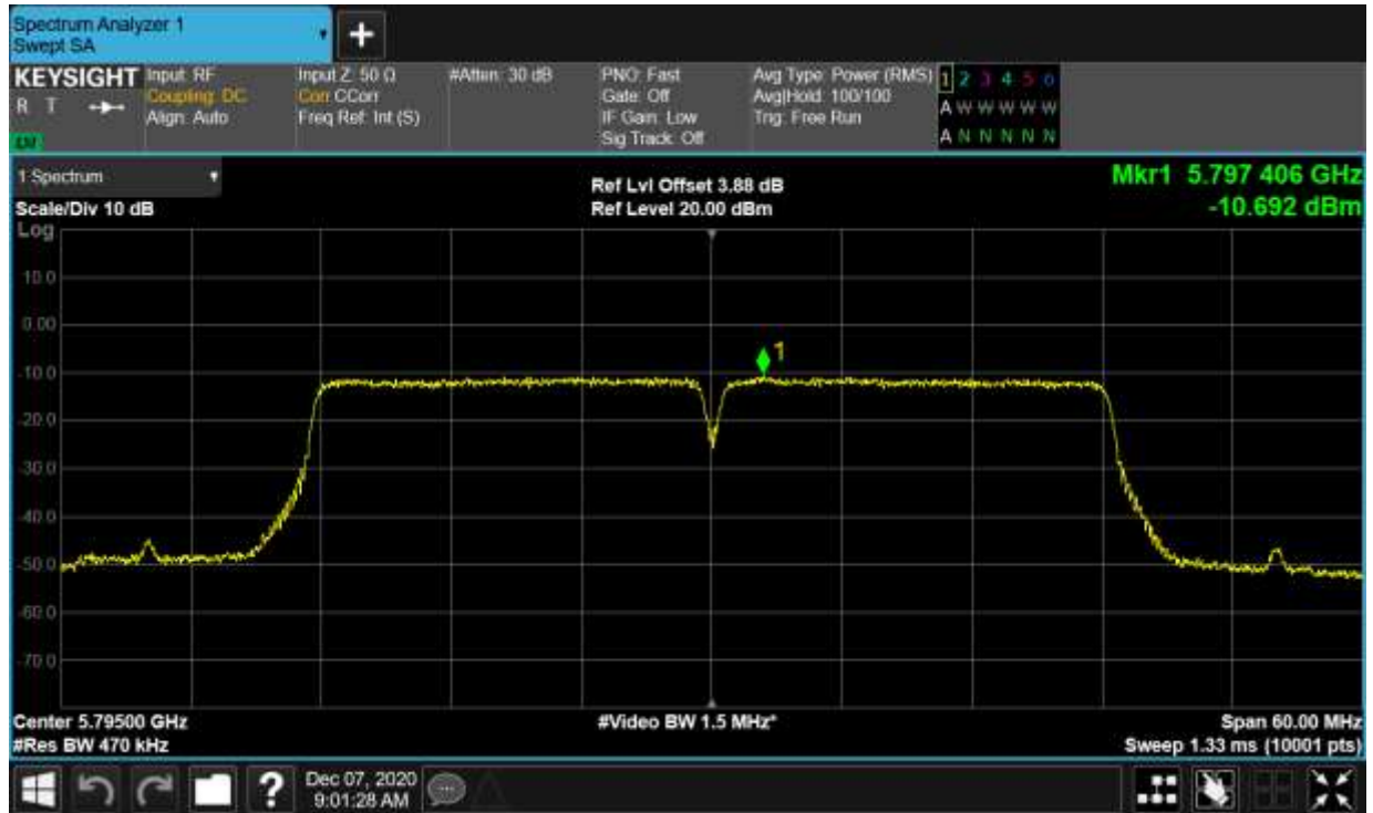
PSD NVNT n20 5745MHz Ant1
