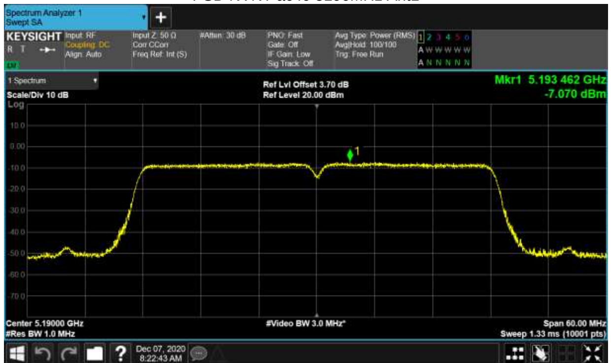
PSD NVNT ac40 5190MHz Ant1
