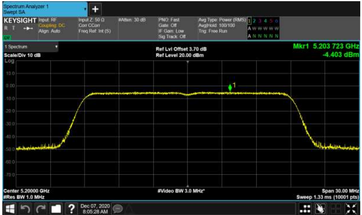
PSD NVNT n20 5240MHz Ant1
