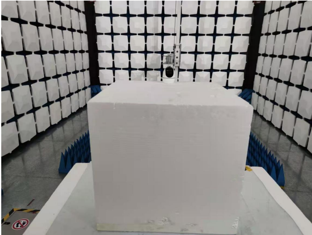
Above 1GHz for radiated emission test setup
