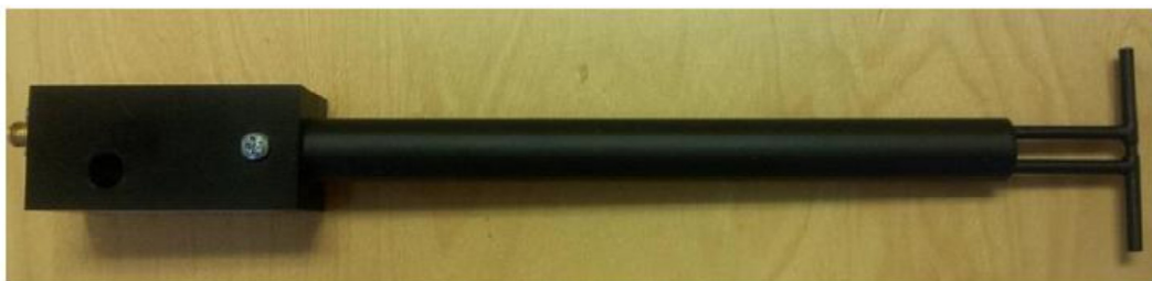
Figure 1 – MVG COMOSAR Validation Dipole
