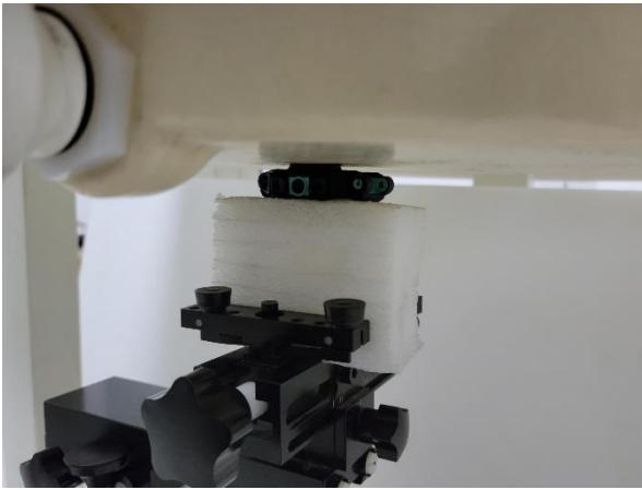
A photograph showing the back side of the EUT positioned 0mm from the back panel. The EUT is mounted on the same black test fixture. The small black device with a digital display is still on top of the EUT. The background is a light-colored wall. |
