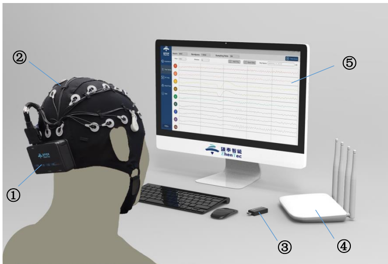
Structure of Wireless Multi-channel EEG Acquisition and Analysis System
