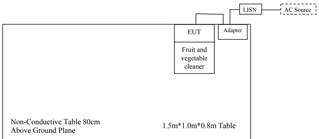
For Radiated Emissions(Below & Above 30MHz):
