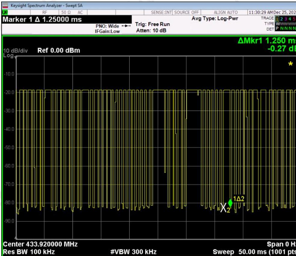
The graph shows the duration of 'on' signal. From marker 1 to marker 2, duration is 650  $\mu$ s.
