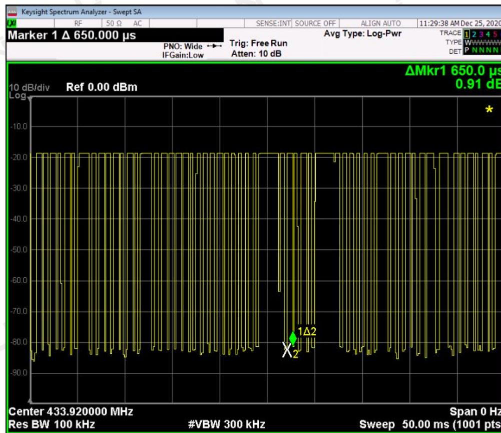
The graph shows the duration of 'on' signal. From marker 1 to marker 2, duration is 350  $\mu$ s.
