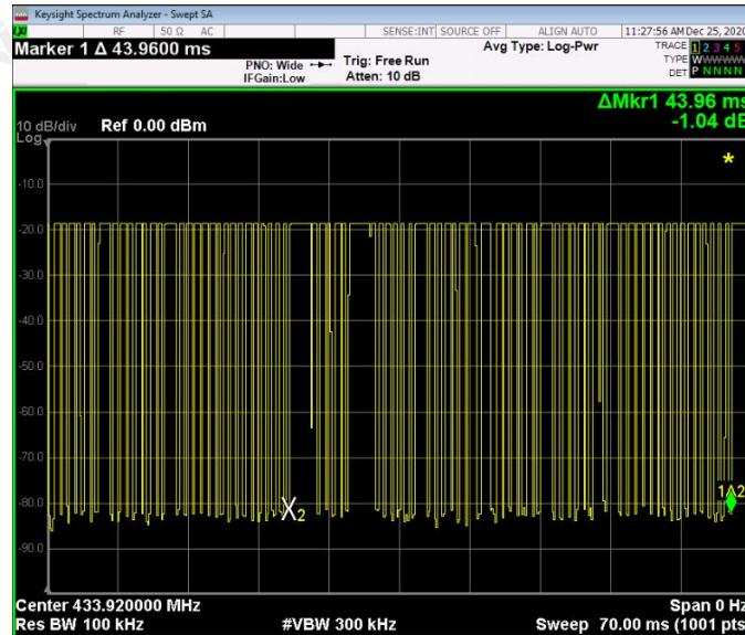
The graph shows the duration of 'on' signal. From marker 1 to marker 2, duration is 2.75 ms.
