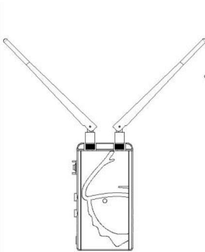
Position the antennas on transmitter and receiver at right angles as shown in the illustration. This ensures the best possible RF performance.
