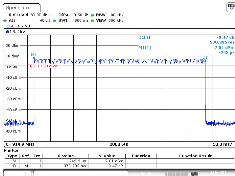
**Hopping Numbers in Observation time (51.8s)**
