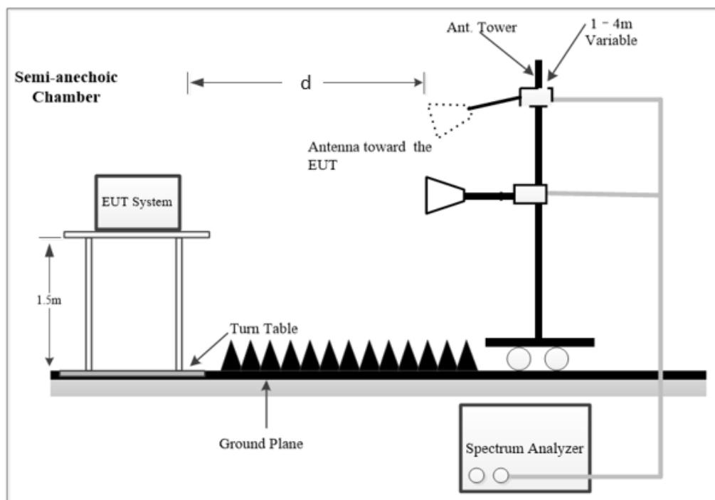
The radiated emissions were performed in the 3 meters distance, using the setup accordance with the ANSI C63.10-2020. The specification used was the FCC 15.209, FCC 15.247 limits.
