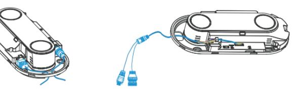
**Note:** If the alarm I/O is going to be used, please connect the Multi-interface to the device.
