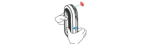
**Note:** Remove the blocking rubber if the wires need to be protruded from the side of the device.
