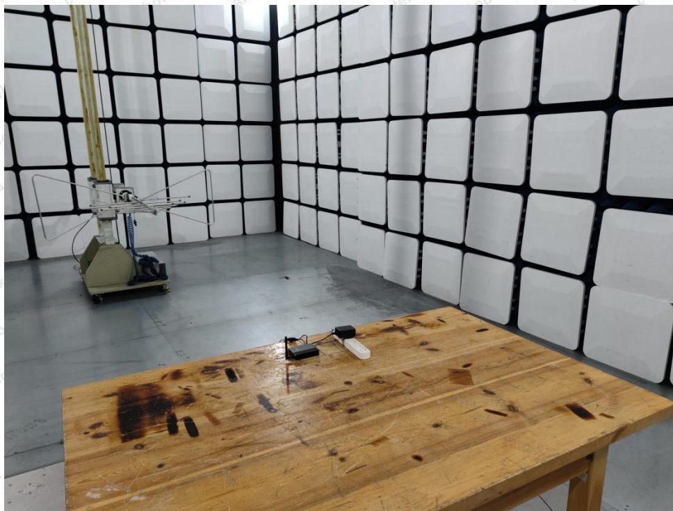
Photo of Radiation Emission Test
