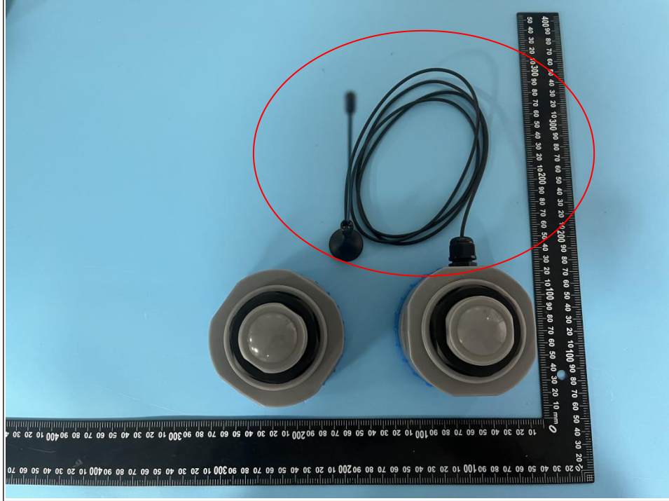
Lora External Antenna
