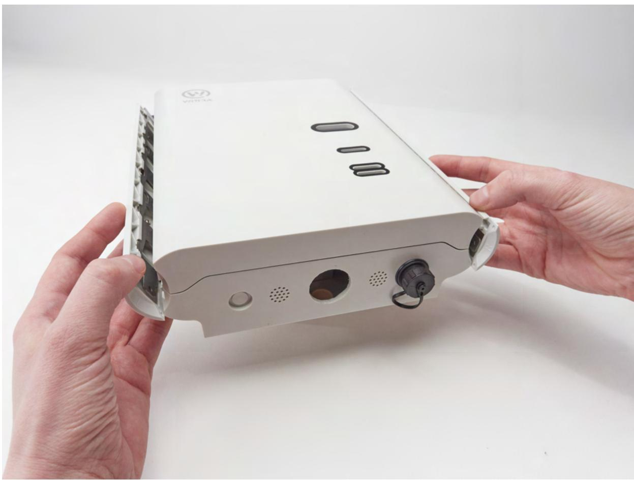
To assemble the gateway casing once again, please note that the side parts are non symmetrical and need to be mounted on the correct side.
