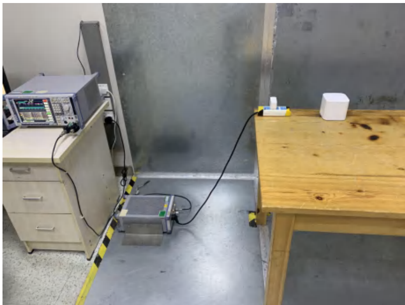
Photo of Conducted Emission Measurement
