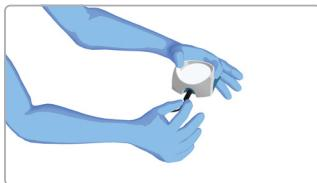
5. Place Izar™ on the docking station. Never place any foreign object, especially metallic, on the docking station as this will prevent Izar™ from being properly charged
