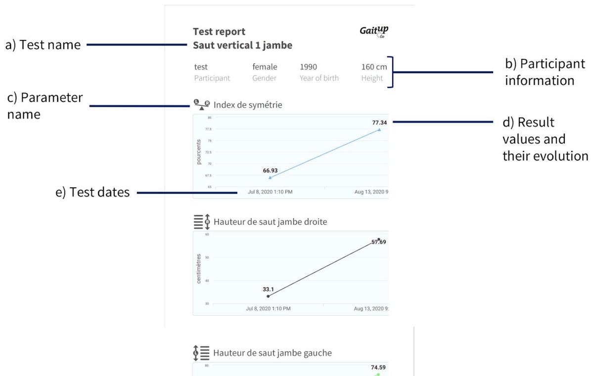
Fig. 86. Comparison report example and its components
