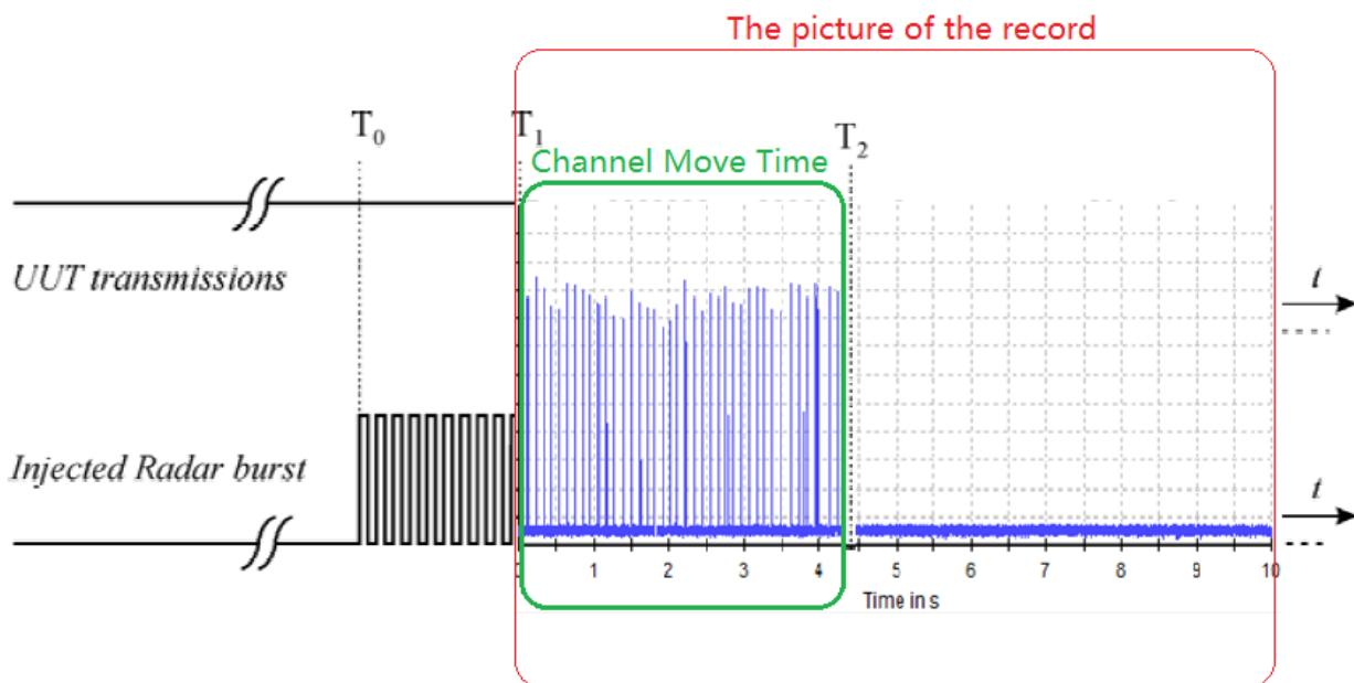
T0 denotes DFS test signal start generated on the channel.
