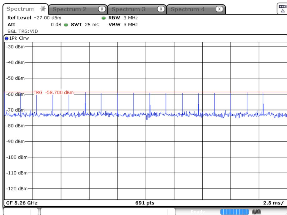
**Radar Type 1 test A Calibration Plot (5260MHz)**
