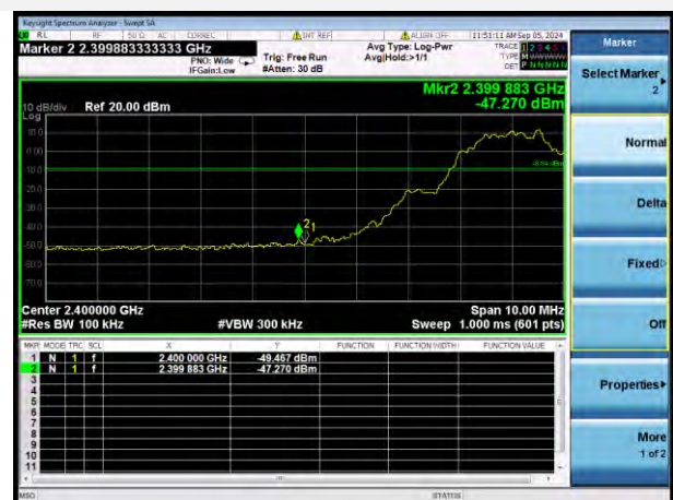
GFSK (BLE 2Mbps) LOW CHANNEL, BAND EDGE
