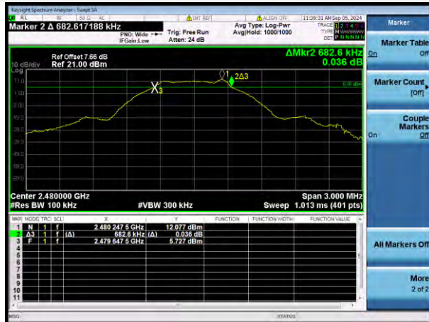
GFSK (BLE 1Mbps) HIGH CHANNEL
