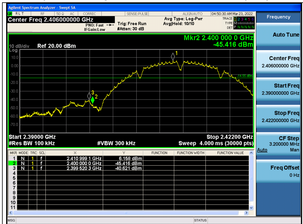
Test_Graph_802.11b_ANT1_2412_1Mbps_Lower Band Edge Emissions
