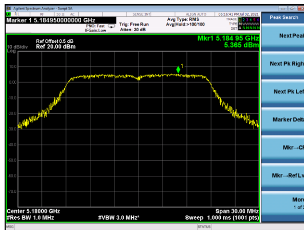
(802.11n20) PSD plot on channel 40
