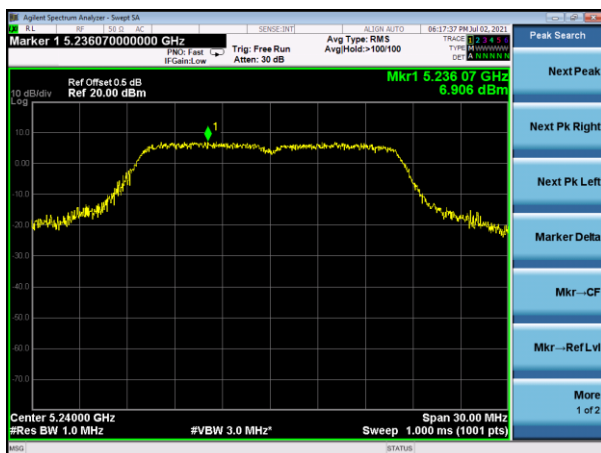
(802.11a) PSD plot on channel 48
