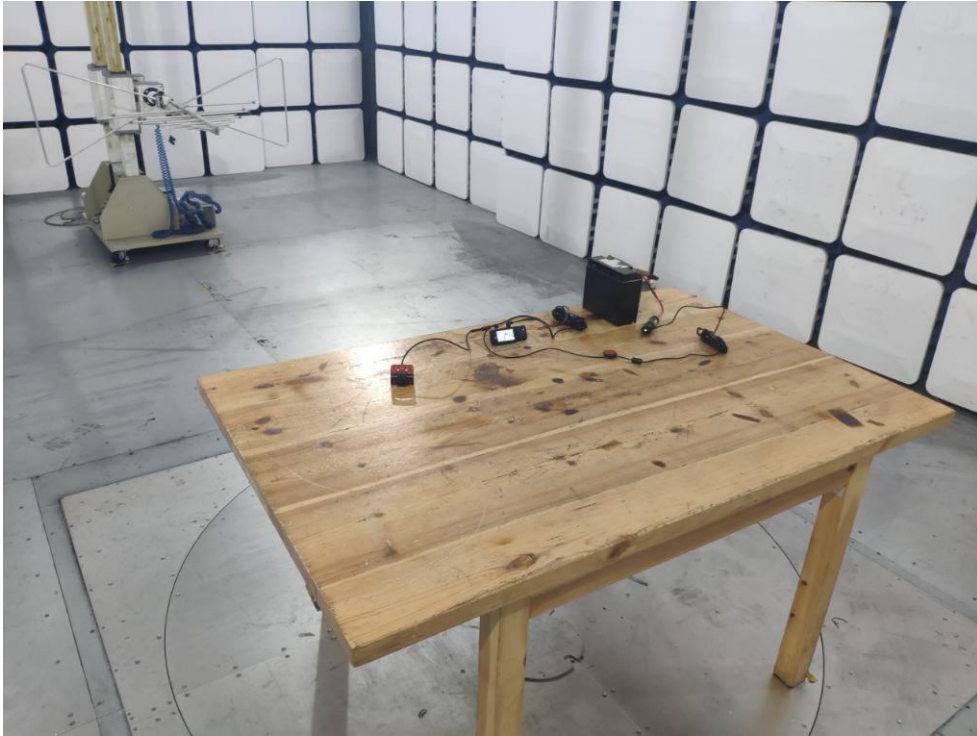
Photo of Radiation Emission Test
