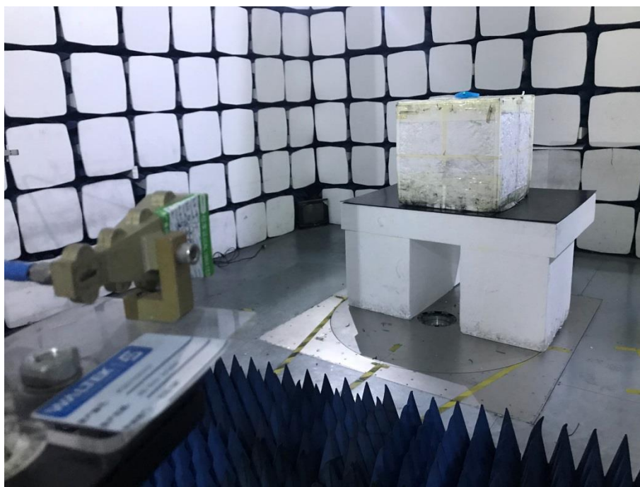
Radiation Emission Test Setup (Above 18GHz)
