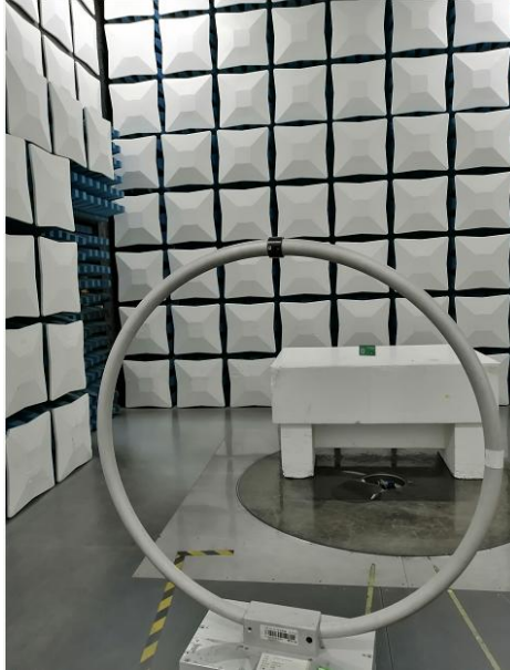
9K-30MHz for radiated emission test setup Model: TP-CCSI-30KW
