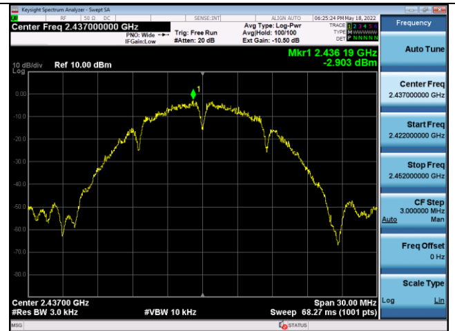
Power spectral density-802.11g ,2412MHz,Ant0
