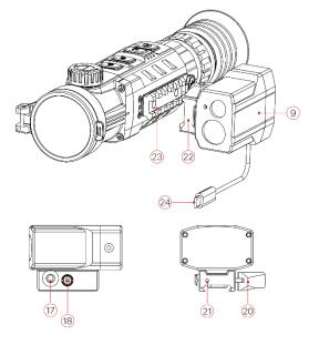
Adjust the hex-nut (18) on the mount (22) to tighten the module (9) using a hex-nut wrench.
