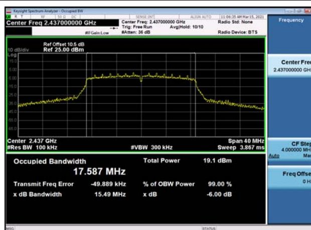
6dB Bandwidth-802.11n(HT20),2437MHz ,Ant0
