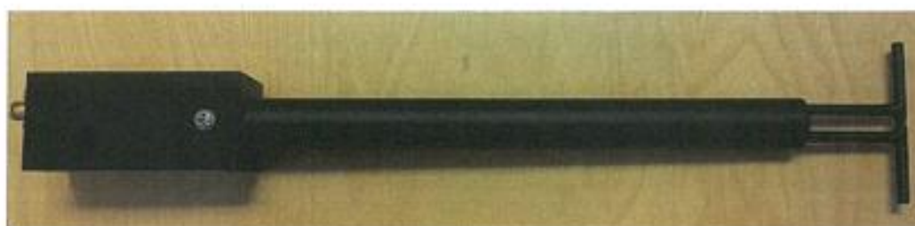
Figure 1 – MVG COMOSAR Validation Dipole
