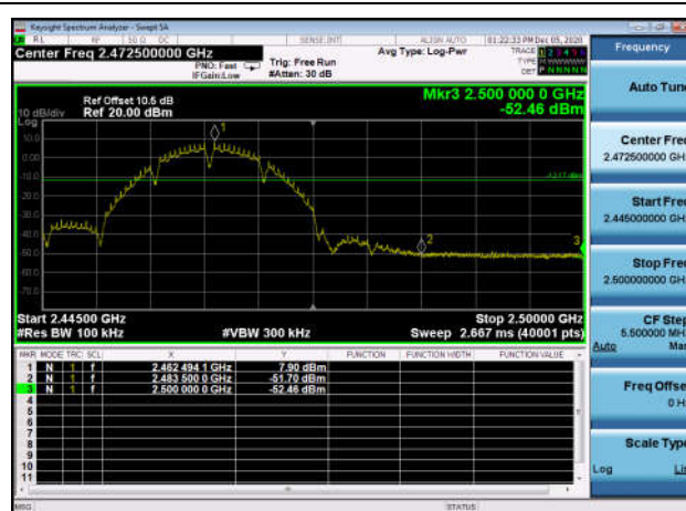
,Plot 2,Band Edge-802.11b,2462MHz ,Ant0
