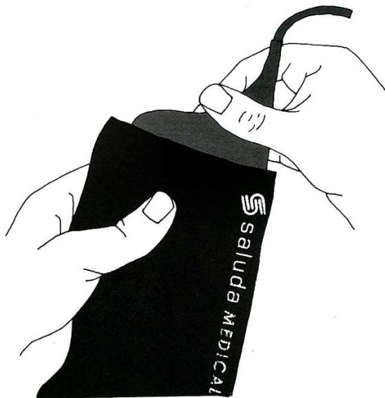
**Figure 9.2: Inserting the Charger coil into the Accessory Belt.**
