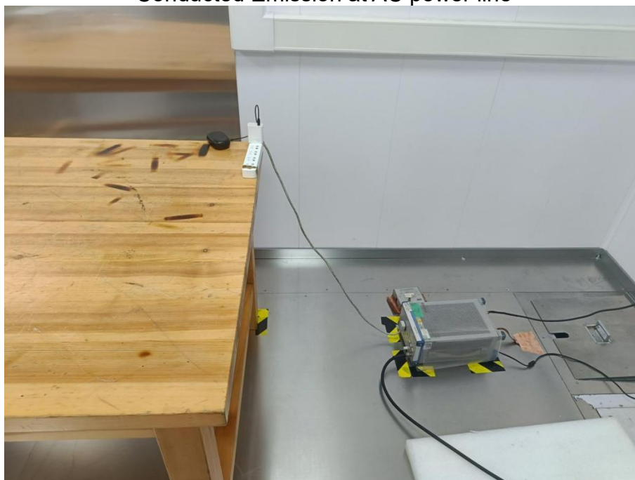
Conducted Emission at AC power line
