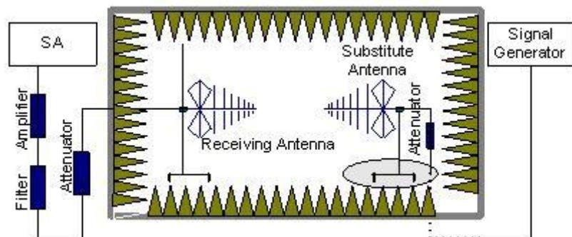
In the chamber, a substitution antenna for the frequency band of interest is placed at the reference point of the chamber. An RF Signal source for the frequency band of interest is connected to the substitution antenna with a cable that has been constructed to not interfere with the radiation pattern of the antenna. A power ( $P_{Mea}$ ) is applied to the input of the
