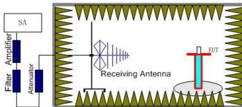
2. The EUT is then put into continuously transmitting mode at its maximum power level during the test. And the maximum value of the receiver should be recorded as (Pr).
