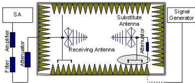
In the chamber, a substitution antenna for the frequency band of interest is placed at the reference point of the chamber. An RF Signal source for the frequency band of interest is connected to the substitution antenna with a cable that has been constructed to not interfere with the radiation pattern of the antenna. A power ( $P_{Mea}$ ) is applied to the input of the substitution antenna and adjusts the level of the signal generator output until the value of the
